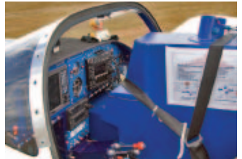
The cramped cockpit, with the overload fuel tank in the right hand seat.
